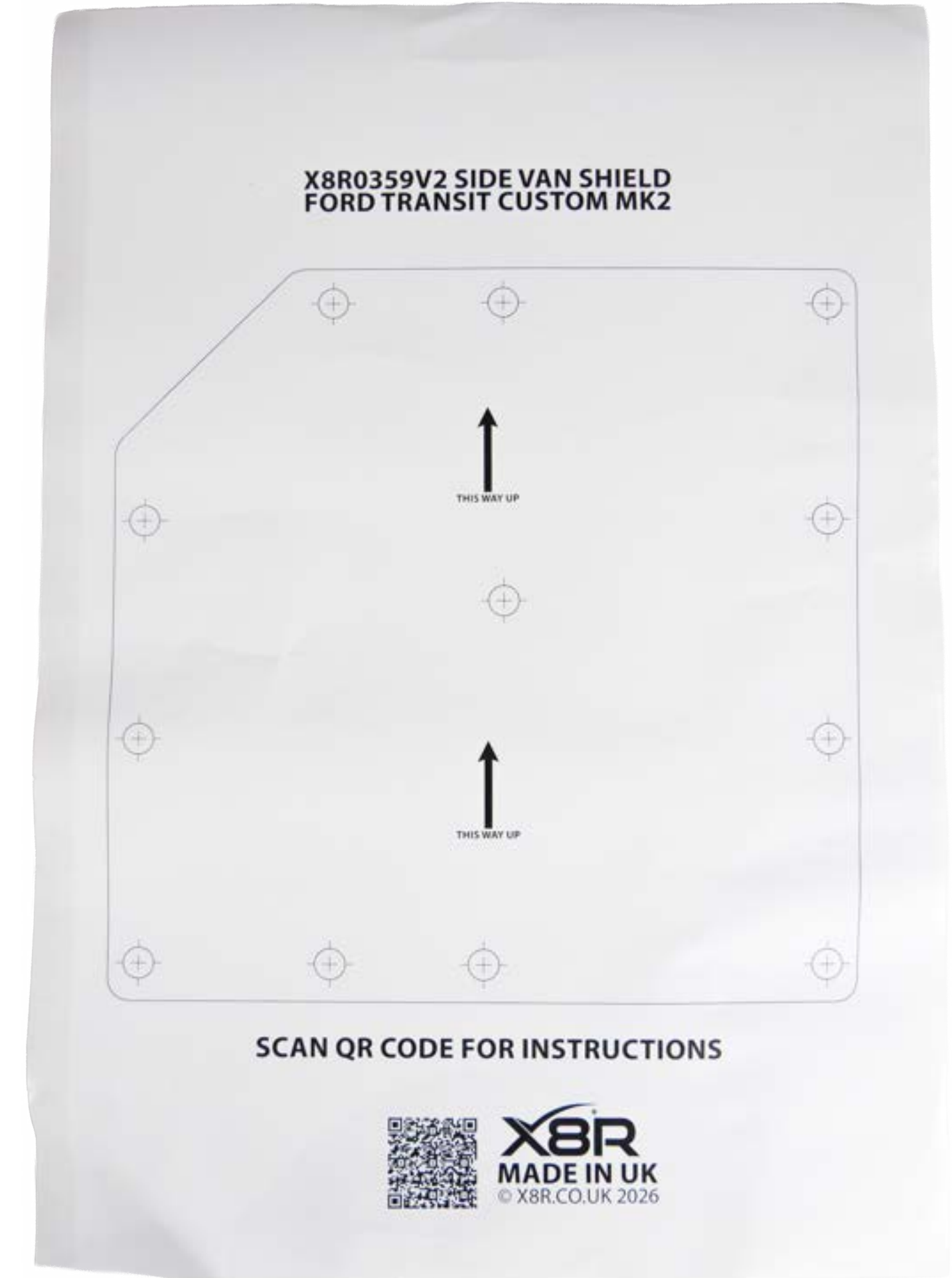
1 Side Drilling Template
