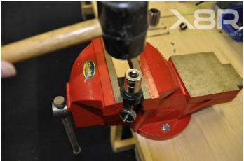
Step 9: Test seal and refit piston
