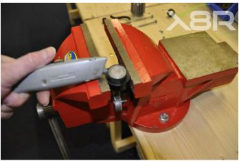
Step 7: Remove seal retaining ring
