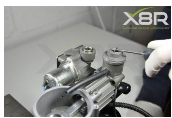
Step 2: Remove compressor head
