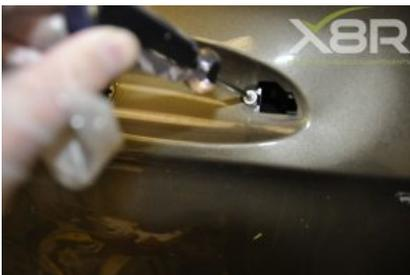
Remove blanking plate and unscrew torx holding outer door handle.
