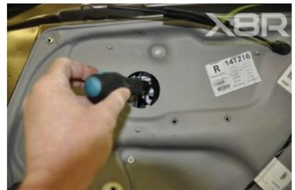
Remove rubber blanks over openings shown.
