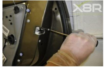
Remove the 3x Torx screws holding the actuator.
