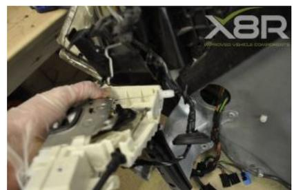
Release electrical connector, linkage and trim to remove actuator from metal
