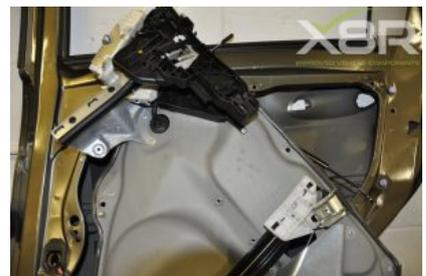
Drill out rivets and remove metal plate. 8 Rivets in total located around the edge of the metal plate.
