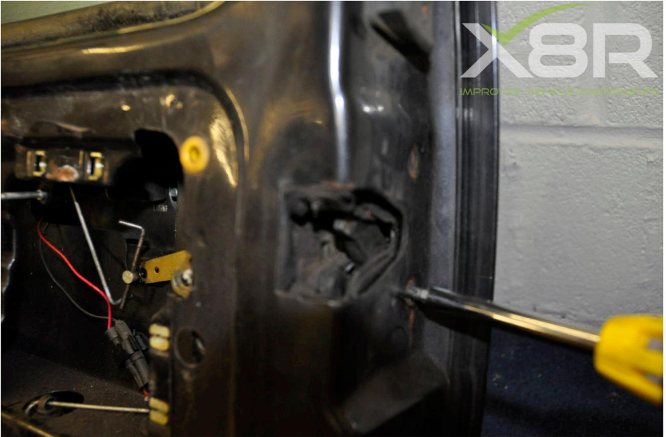
Remove screws retaining lock mechanism.
