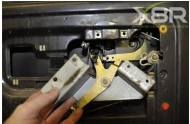
Remove pivot point which prevents door lock mechanism removal.
