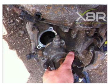
Step 2: Remove worn pivot pin.
